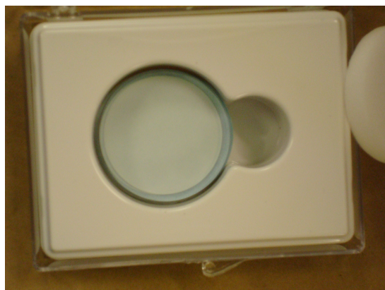
Figure 2.3 Top view of commercially available alumina membrane (Whatman Corp, Britain).
