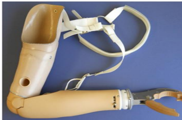
Figure1.2 Body-powered prosthesis: The harness captures the user's motion and transfers this movement through the cable to control the terminal devices (Behrend et.al. 2011)
