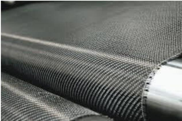
*Figure 3-2 Carbon-Epoxy*
