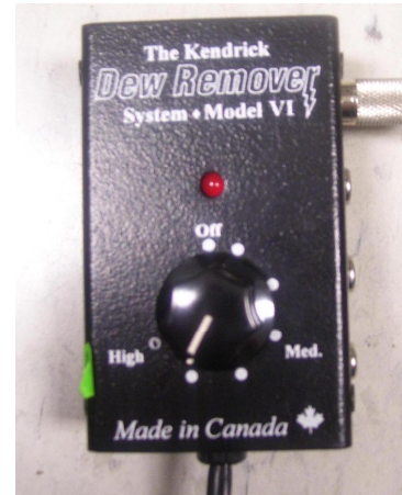
Figure 2.8: Picture of the Temperature Controller. This Controller is used to regulate the temperature inside the environmental chamber. It has a dial to select OFF, MED, HIGH modes of temperature control.
