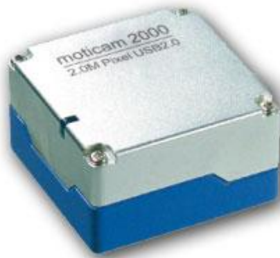
Figure 2.9: Picture of the Motic Moticam 2000 Camera adapted from [80]. The Motic Moticam 2000 camera is encased in light weight aluminum and has a USB connecting cable to connect to the computer.
