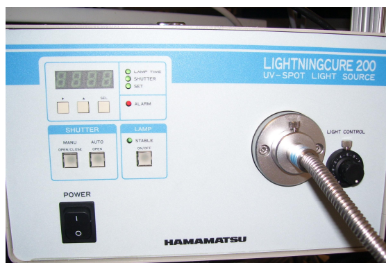
Figure 2.2: Hamamatsu LightCure UV Spot Light Source. It contains a 200W HgXe lamp and a reflector for the UV. The quartz fiber guide carries the UV light from the lamp to the next set of optical components.
