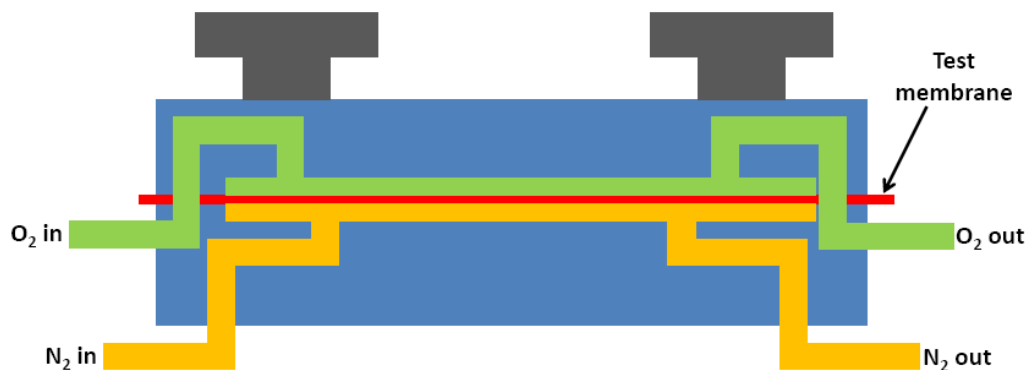
Figure 3.16. Cross-section of oxygen transmission rate test chamber.
