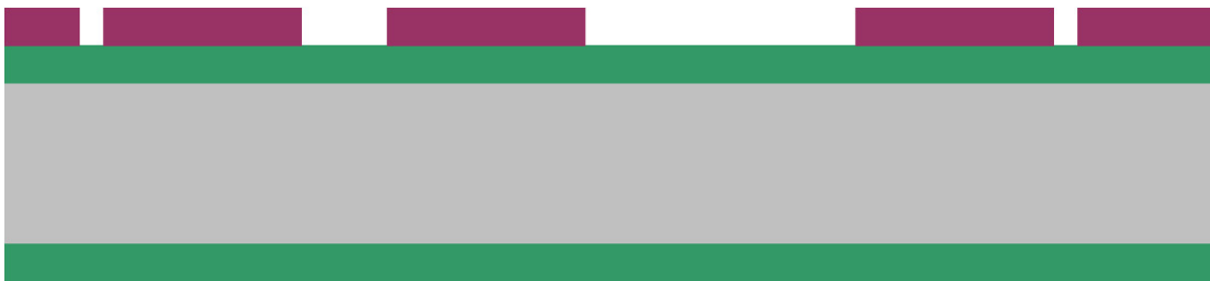
Figure A.2. Corss-section of wafer after Lithography.
