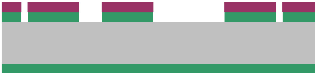
Figure A.3. Cross-section of wafer after patterning the nitride using DRIE.
