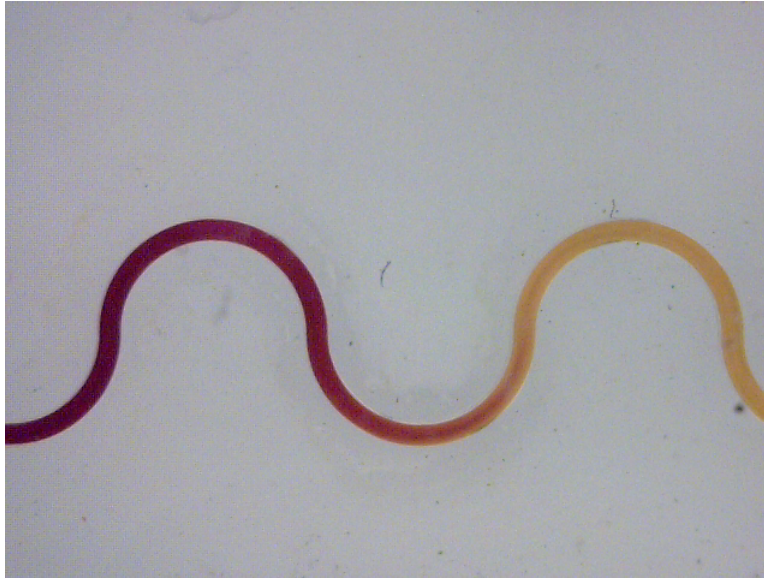
Figure 3.32. A close-up view of pH color change zone.
