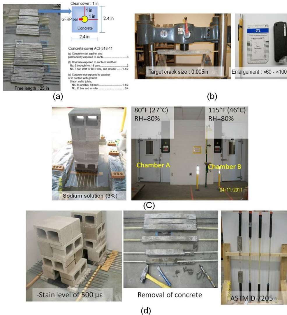
Figure 4.1 (a) Fabrication of tensile specimens embedded in cement mortar paste (b) Initial cracks (c) Simulation of the chemical environment (saline) (d) Sustained loading at Chamber and steel grip based on ASTM D7205
