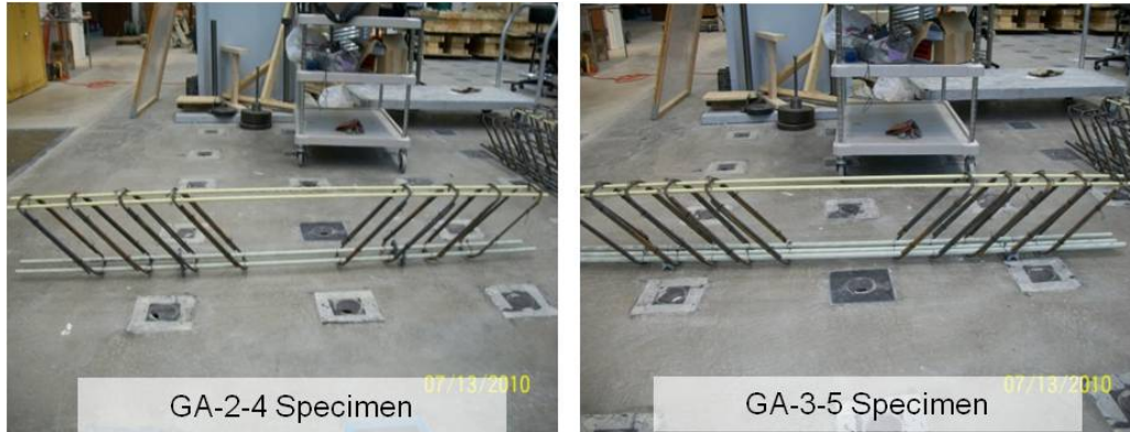
Figure 6.2 Reinforcement caging for each case ( GA-2-4 and GA-3-5 )
