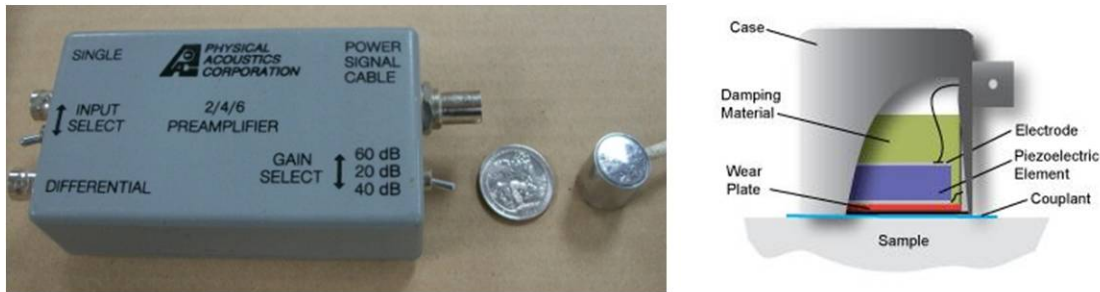
Figure 8.2 Pre-amplifier and a sensor used for acoustic emission evaluation ( www.ndt-ed.org )
