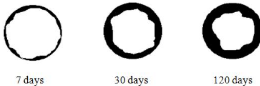
Figure 3.1 Rough estimate of alkali penetration in GFRP rods (Katsuki and Uomoto, 1995)
