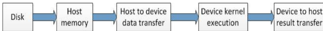
Figure 3.17 Overview of GPU application showing data copying from host to GPU memory, launching GPU kernel, and copying results back to the CPU memory. Reprinted by permission from Elsevier [168]
