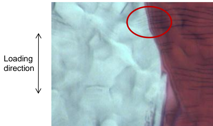
Figure 5.14: Micro-cracks development at marked area.
