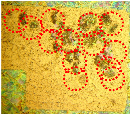
Figure 4.22 Peeling of wire bonding pad by wire bonder capillary.
