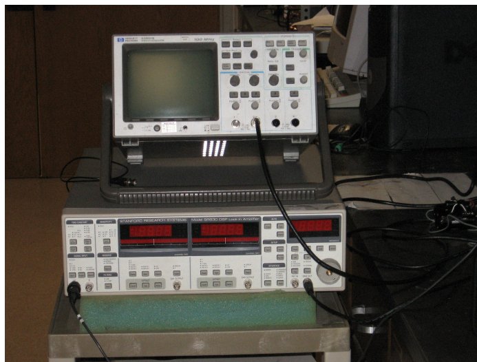
Figure 2.6 Oscilloscope for the acceleration (top) measurement and Lock-in amplifier for voltage (bottom)
