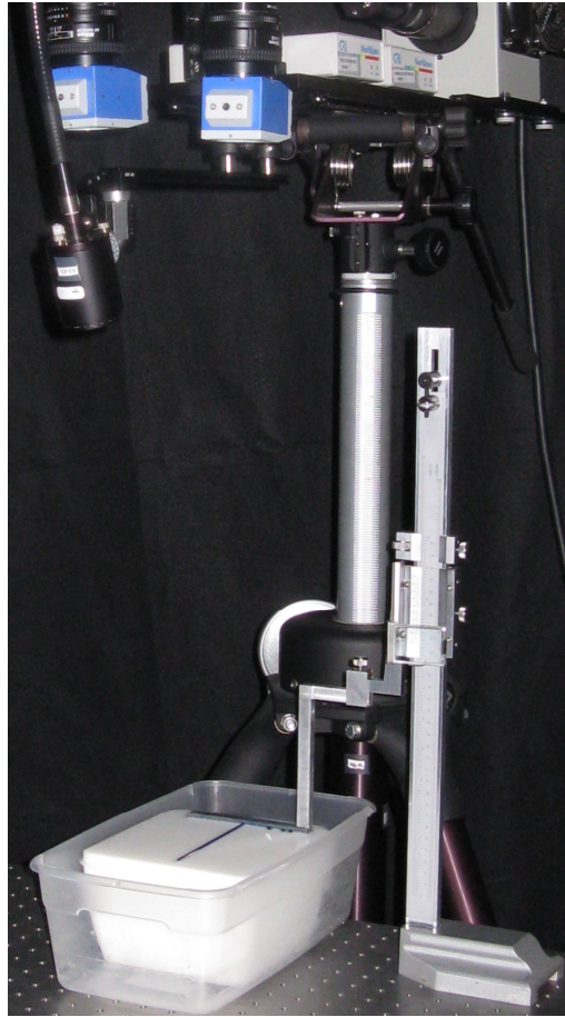
Figure 21. Experimental set up of the multimodal hyperspectral imager for acquiring images of the intralipid phantom model
