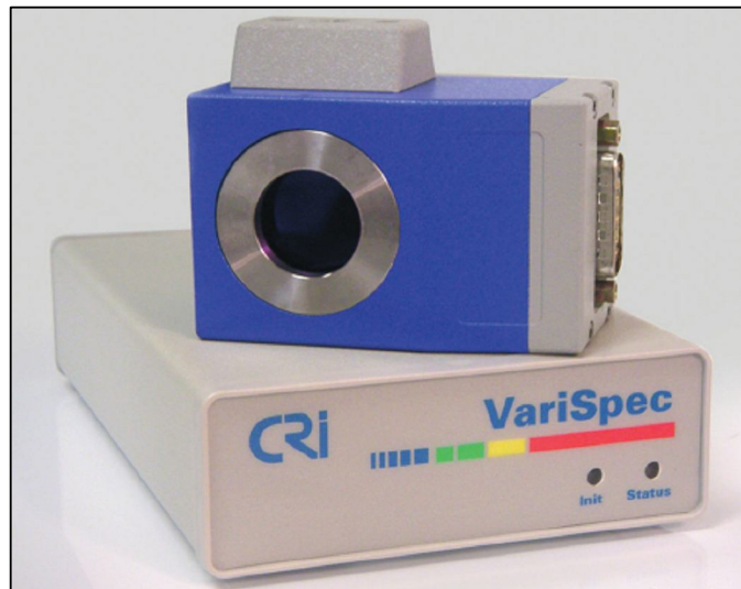
Figure 4. LCTF module comprising of the LCTF and the control box [15]
