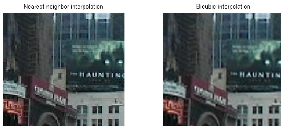
Figure 4.2 (a) Original image on left panel and its top right cropped image on the right panel. (b) Interpolation of the cropped image using nearest neighbor (left panel) and bicubic (right panel).
