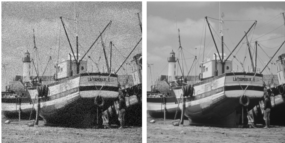
Figure 1.3 Example of the noise-corrupted image (left panel) of an original scene (right-panel)
