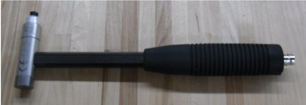
Figure 4.7 PCB Impact Hammer.
