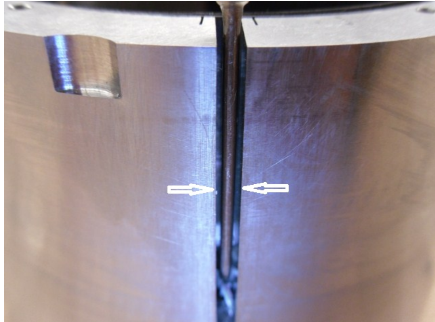
Figure 3.12 Orifice Tube Interference with Bearing Sleeve.
