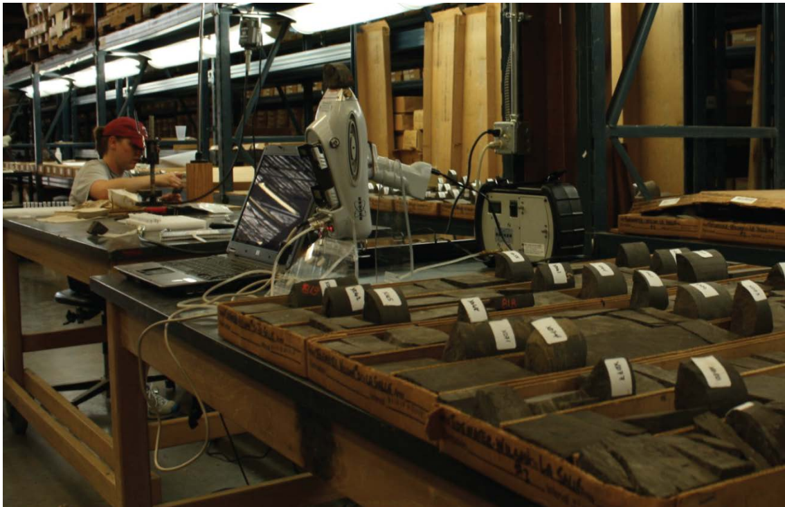
Figure 2.2 Picture of a Bruker Tracer III-V handheld ED-XRF spectrometer that was utilized for geochemical analysis. Note: 2/3 section of slabbed core sitting atop spectrometer aperture.
