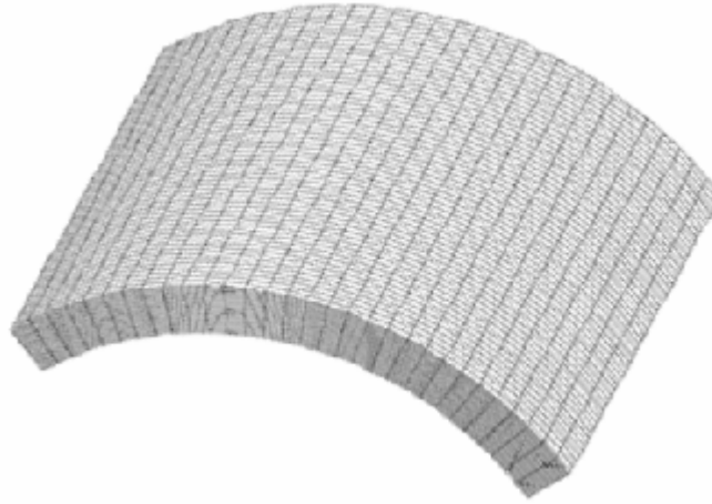
Figure 3. Representative model of a simply curved composite laminate with regular cubic mesh with each cubic mesh consisting of a finite element [6].
