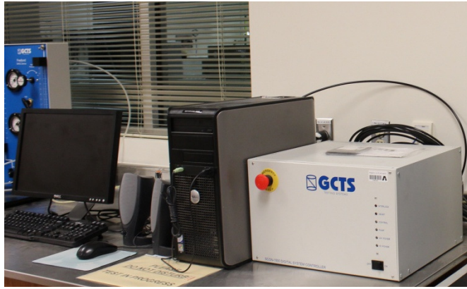
Figure 3.30 Data acquisition and process control system
