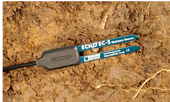
Figure 3.13 EC-5 soil moisture sensors
