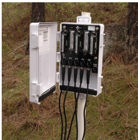
Figure 3.16 Em-50 Data logger
