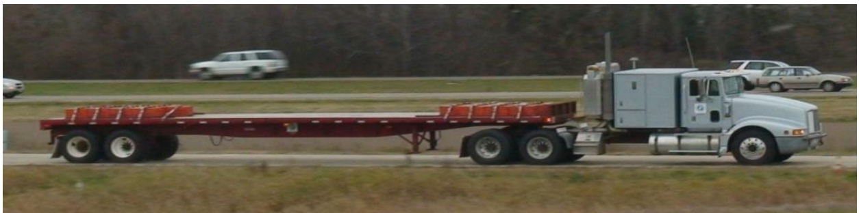
Figure 3.5 The 80K truck used in LVR for loading
