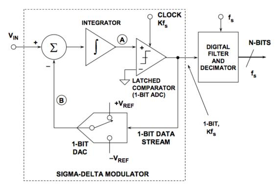
Figure 2.9 Sigma-Delta ADC Architecture
