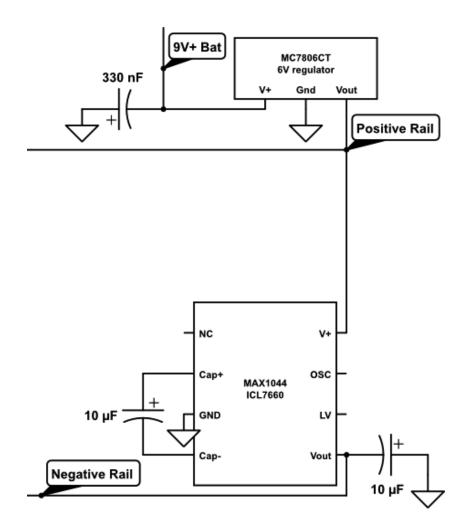
Figure 5.7 ECG Power Circuit Diagram
