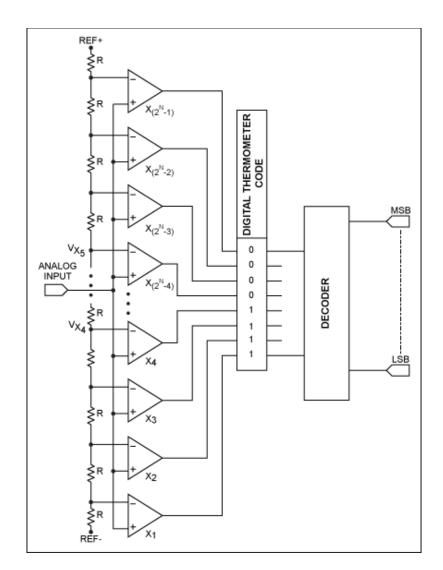
Figure 2.8 Flash ADC Architecture
