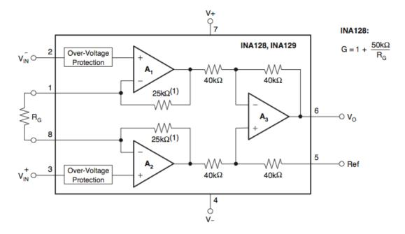
Figure 5.2 INA128 circuit diagram
