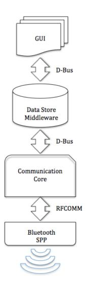
Figure 8.1 Server Unit Block Diagram
