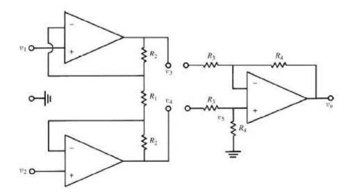
Figure 2.7 3-Opamp Instrumentation Amplifier
