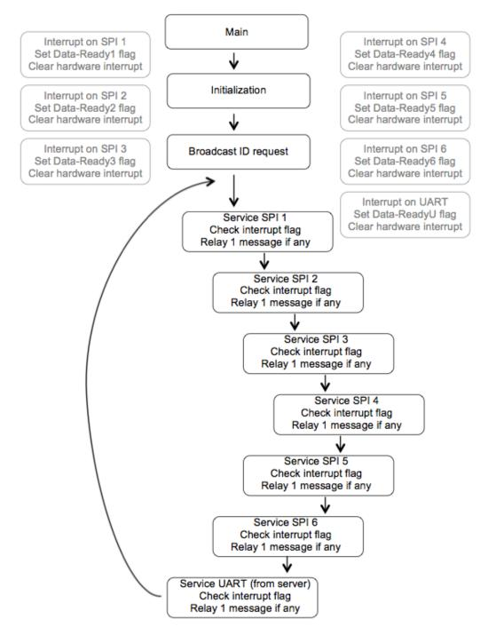
Figure 4.5 Core Unit's Program Flow
