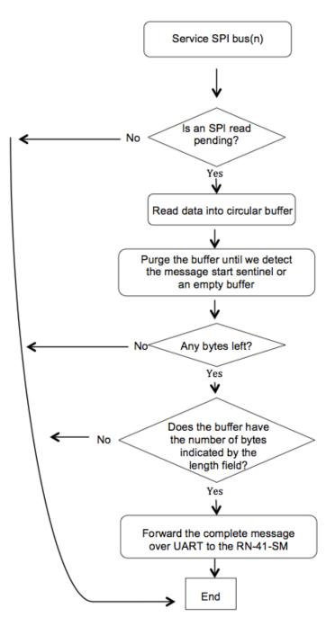
Figure 4.6 Service SPI bus program flow
