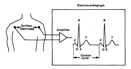
Figure 2.6 Image of a typical electrocardiograph
