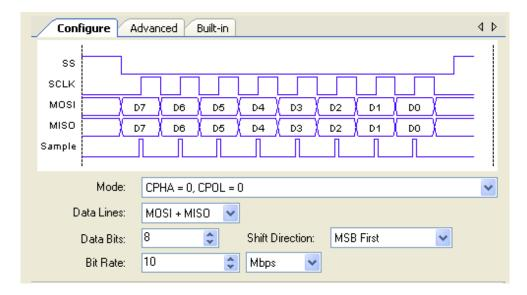
Figure 4.3 SPI slave configurations
