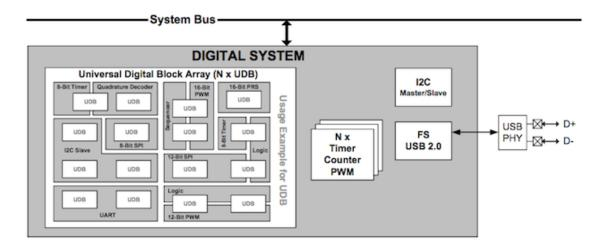
Figure 2.10 PSoC 5 digital system block diagram
