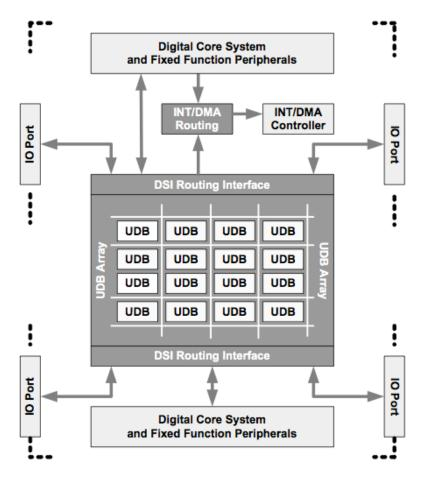
Figure 2.11 PSoC 5 digital system interconnect (DSI) diagram
