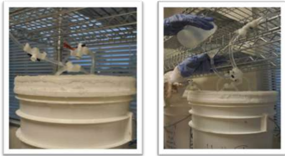
Figure 3.6: Water Addition for Rainfall Simulation
