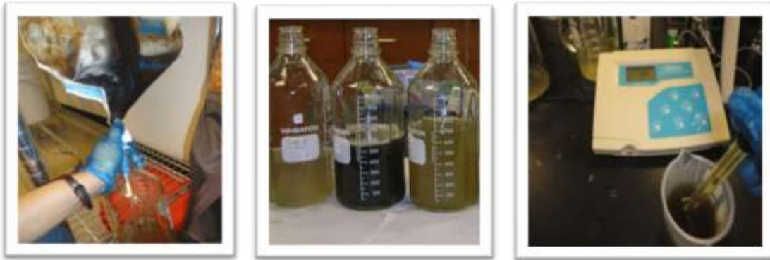
Figure 3.8: Leachate Collection, and pH Measurement Procedure
