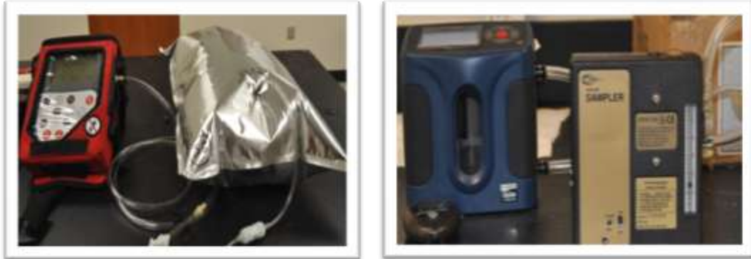
(a) (b) Figure 3.7: Gas Measurements (a) Composition using Landtec GEM 2000 and (b) Volume using SKC Sampler & Calibrator
