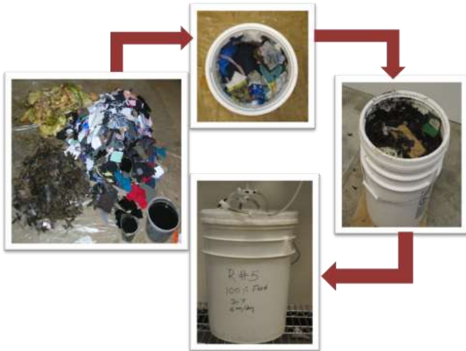
Figure 3.5: Reactor Installation Process
