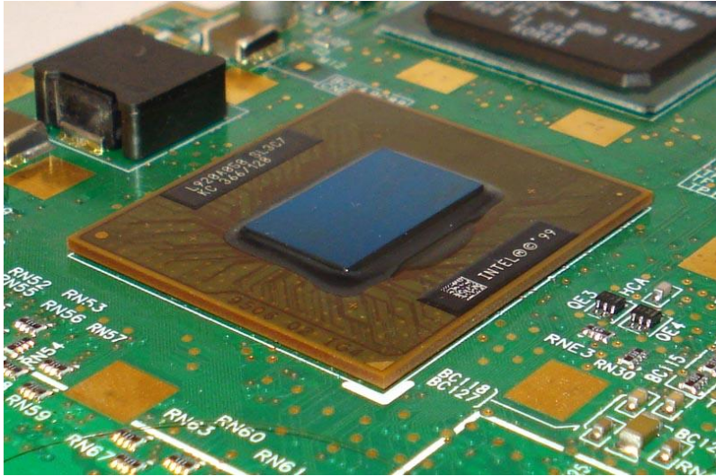
Figure 6.2 Intel mobile celeron in a BGA2 package (FCBGA-479) [38]
