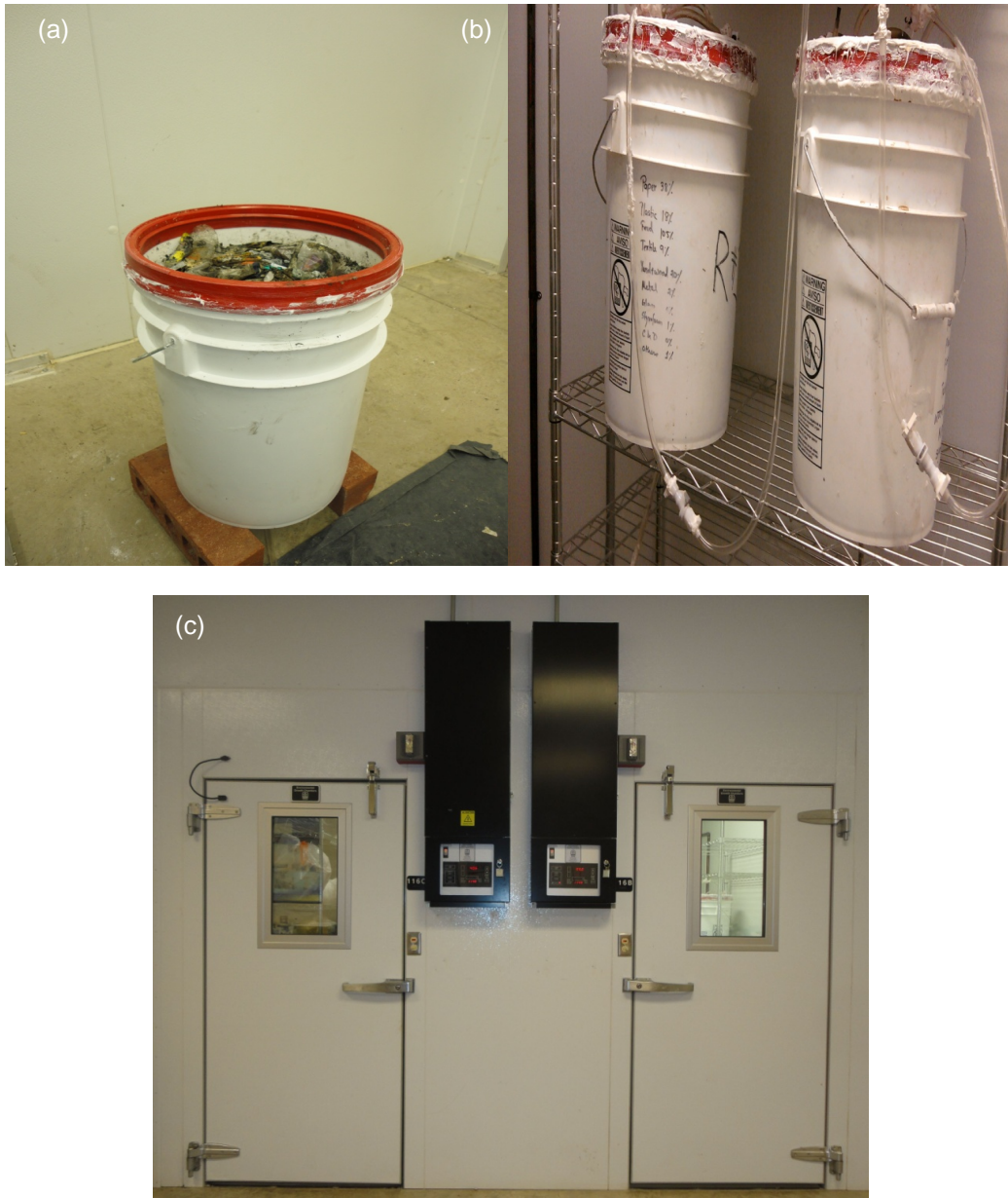
Figure 3.10 Reactor set up (a) Reactor Filling (b) Reactors in Operation and (c) Environmental Growth Chambers
