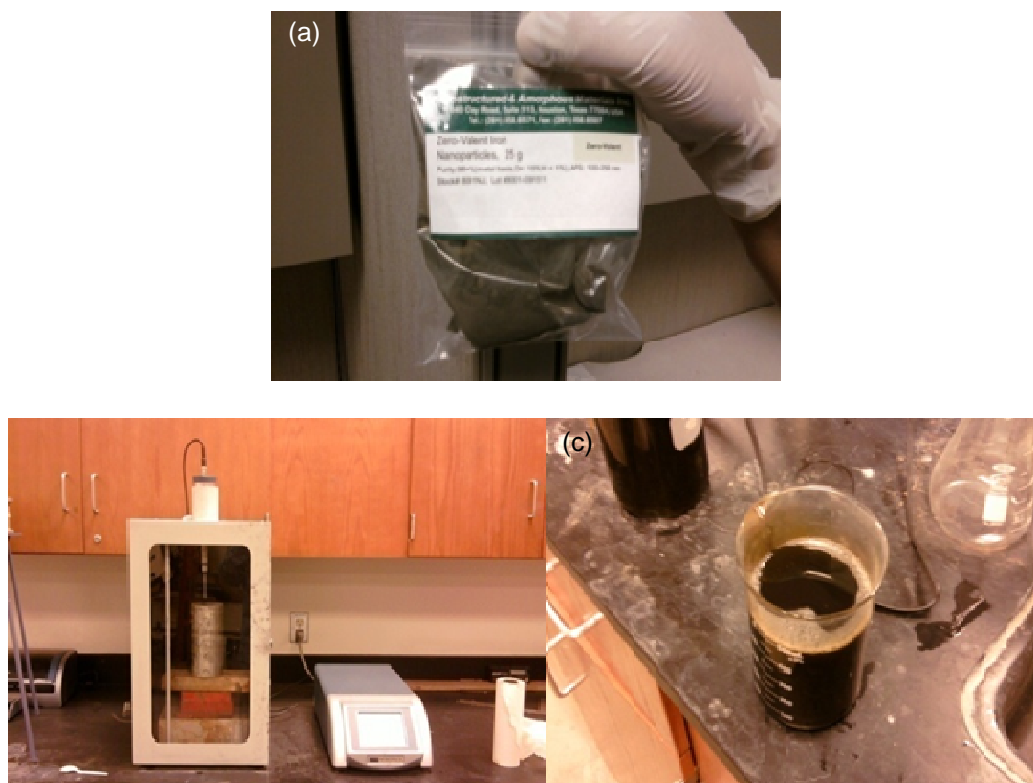
Figure 3.13 Sonication (a) Powdered nZVI (b) Sonicator and (c) Sonicated nZVI in water
