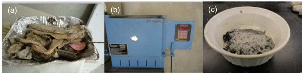
Figure 3.7 Volatile solids test (a) Dry Sample (b) Muffle Furnace and (c) Burnt Sample
