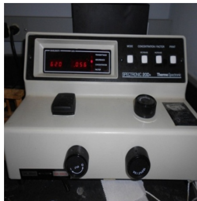
Figure 3.20 Spectrophotometer for Absorbance Measurement
