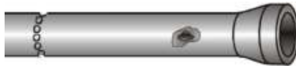
Figure 2.1 Corrosion Failures (Makar et al., 2001)
