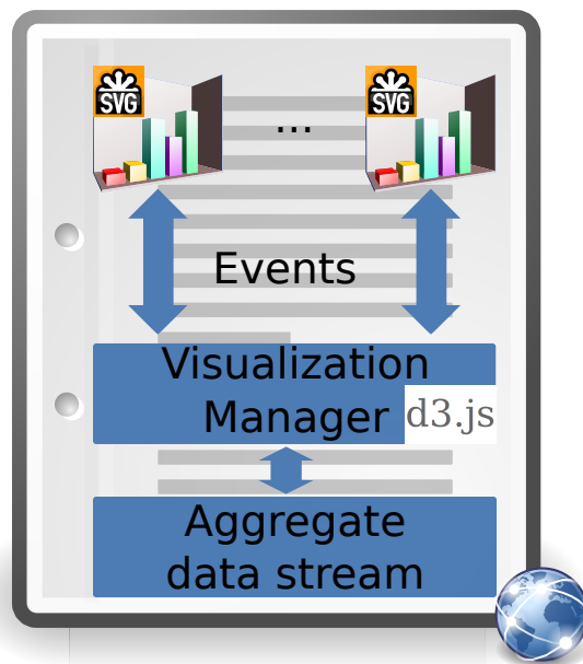
Figure 6.4. Architecture of data visualization subsystem. Aggregate data are visualized on SVG-based charts and maps using JavaScript and D3. A JavaScript-based visualization manager processes user-generated events such as panning and zooming and brush-and-linking, and updates the visualizations accordingly.
