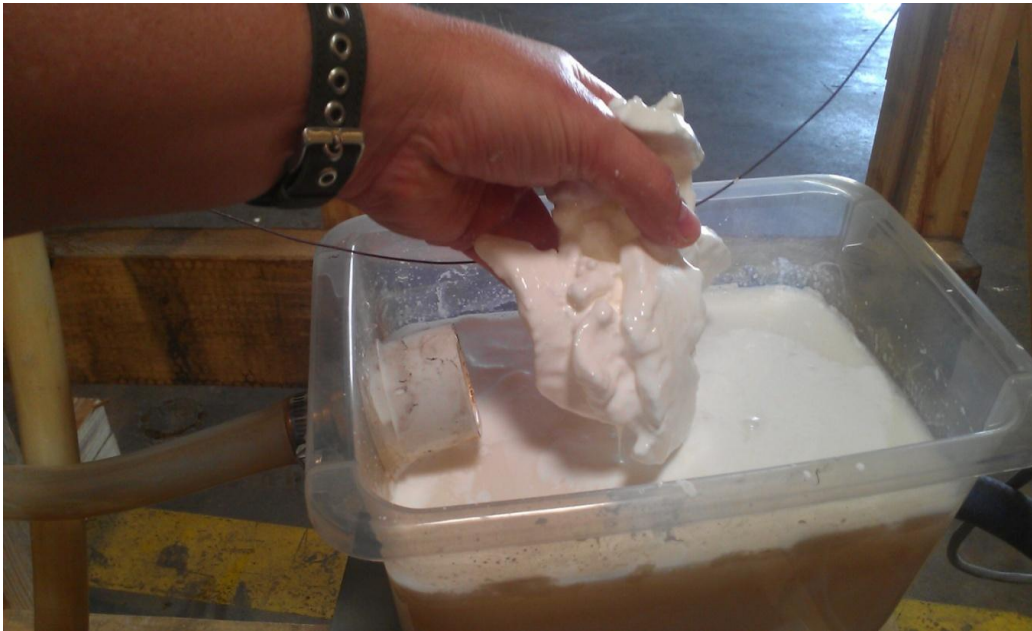
Figure 5.7: Agglomerate of mPCS in Expansion Tank
