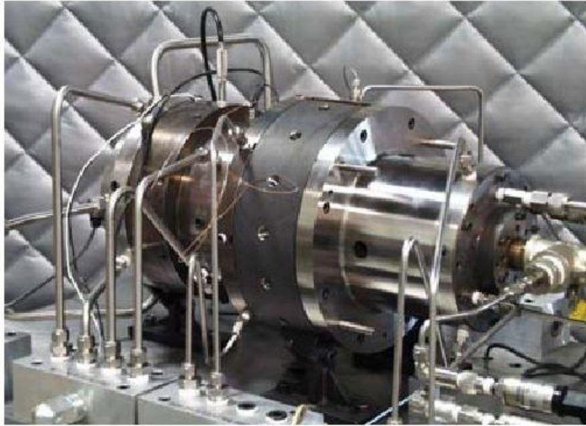
Figure 2-5 Foil Thrust Bearing Rig, image from [6]
