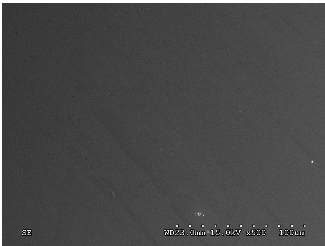
Figure 5.22: Surface morphology of nc Ni sample after open circuit potential vs. time measurement in aerated 3.5 % NaCl solution.
