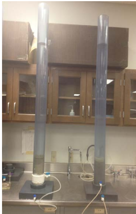
Figure 3.11 Combined Device with Leachate Apparatus.
