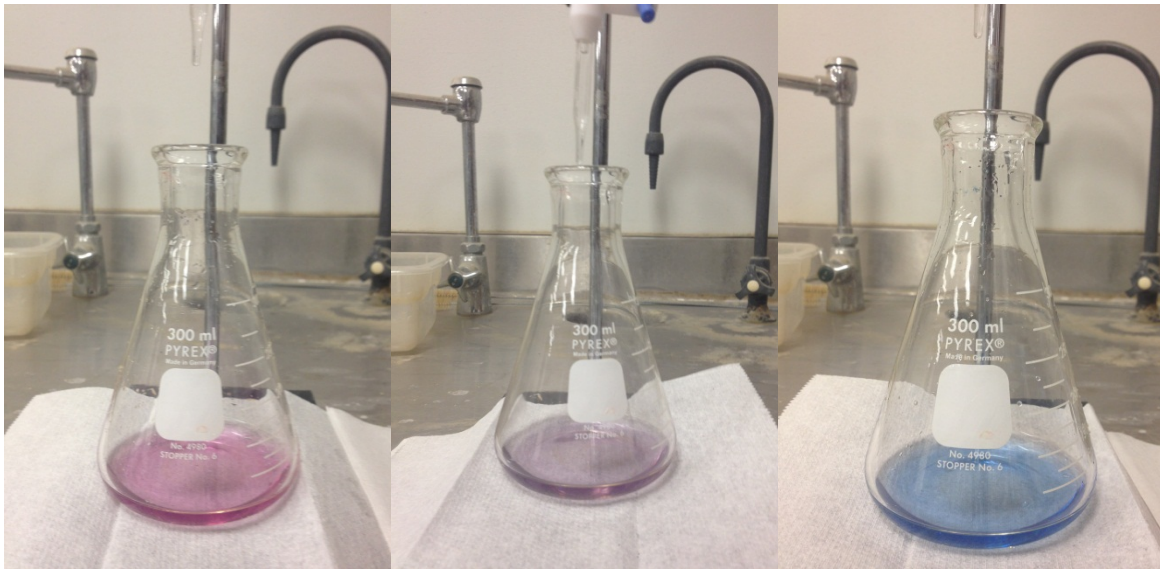
Figure 3.13 Showing EDTA titration stages (a) Represents Starting point. (b) Represents the color change before endpoint (c) represents the end point.
