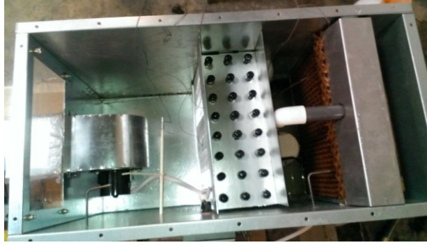
Figure 5.9: Placement of mPCM Coils in Evaporative Cooler
