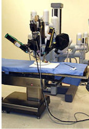
Figure 1.1. da Vinci Surgical System Manufactured by Intuitive Surgical used in Surgeries via Minimally Invasive Approach (MIS) (Image Courtesy: www.absoluteastronomy.com ).
