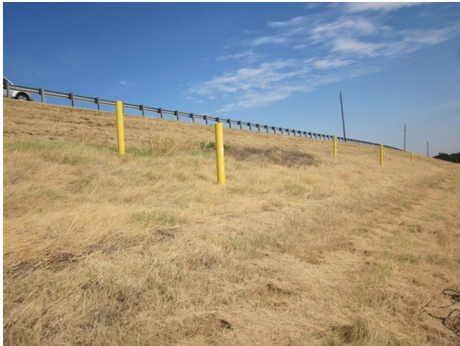
Figure 4.62. Vegetation on 4%lime + 0.3%fiber, 8%lime + 0.15%fiber and 8%fiber sections (Joe Pool Dam)
