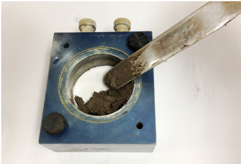
Figure 3.6. Placement of soil paste into the shear box
