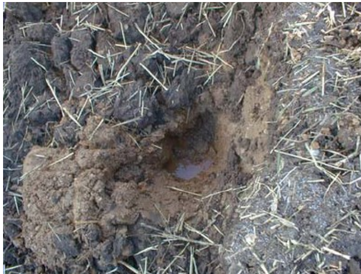
Figure 2.48. Perched water on a failure surface through seepage (Titi and Helwany, 2007)
