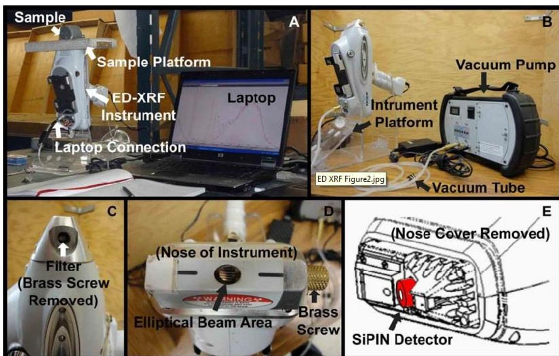
Figure 2.1 Instrument setup (A) Showing the general setup (B) illustrating the the vacuum pump and platform (C) filter loading area (D) 3x4 mm beam area (E) SiPin Detector (Hughes, 2011).
