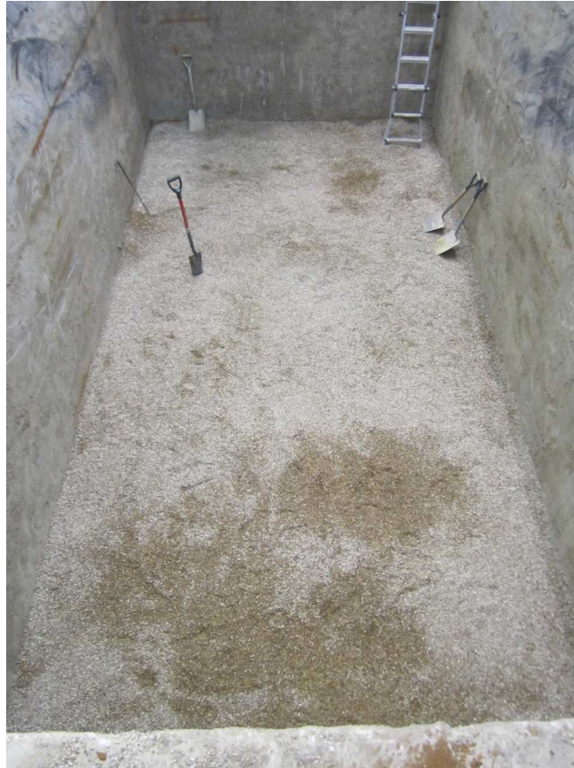
Figure 3.2: Soil Box with Bedding Layer for Test 1
