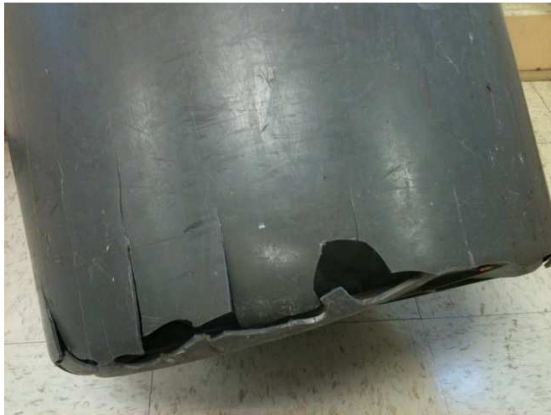
Figure 4.12 Cracked Trash Can
