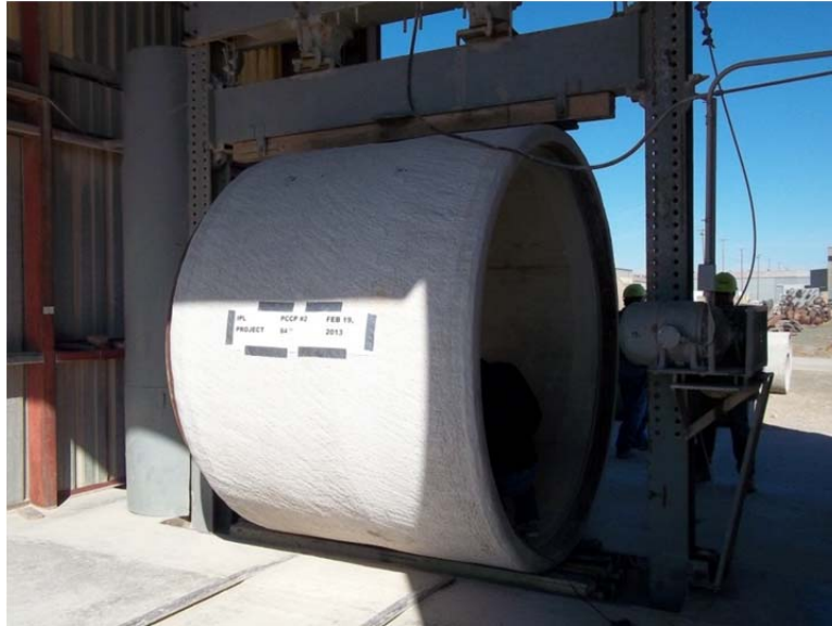
Figure 2.7 PCCP-ECP placed on testing machine
