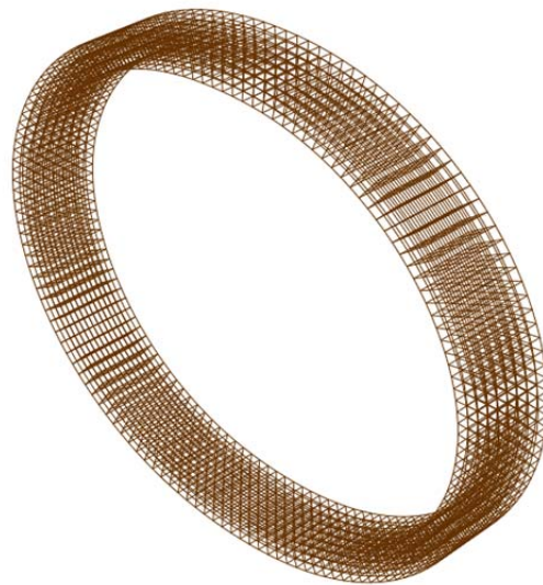
Figure 3.4 Converged mesh of concrete core
