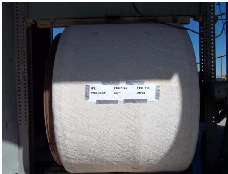
Figure 2.3 PCCP-ECP on three-edge bearing testing machine
