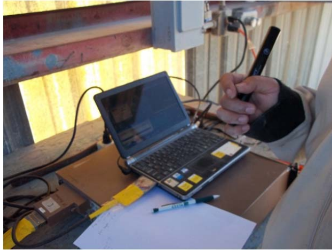
Figure 2.10 Connection of CDS and load cell to Vishay scanner
