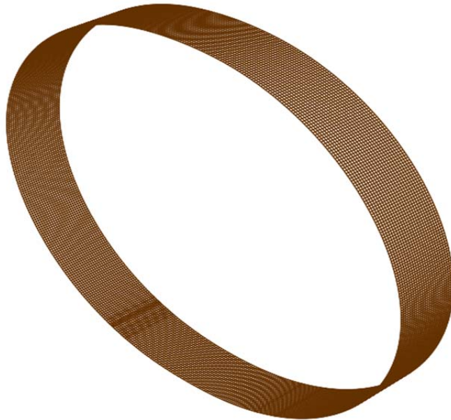
Figure 3.6 Converged mesh of steel cylinder
