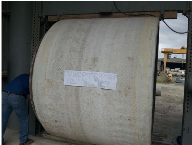
Figure 2.9 Top bearing brought in contact with PCCP-ECP
