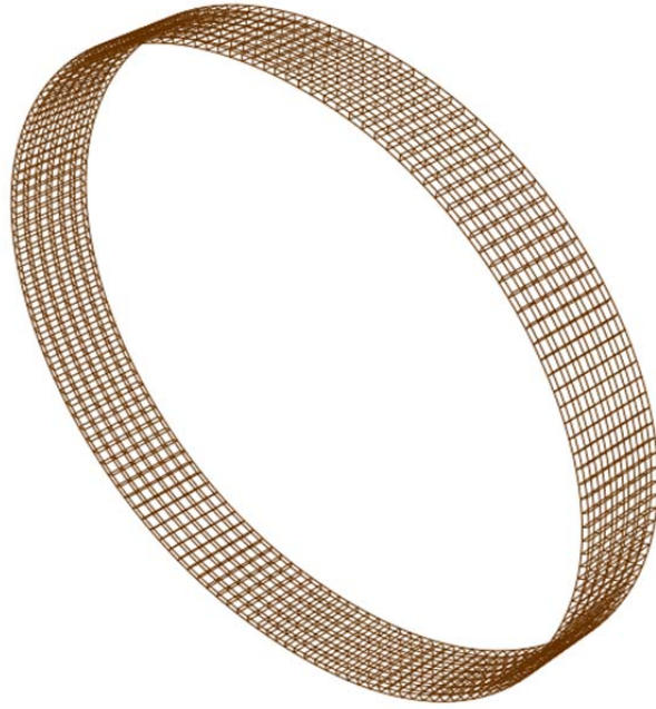
Figure 3.5 Converged mesh of mortar coating
