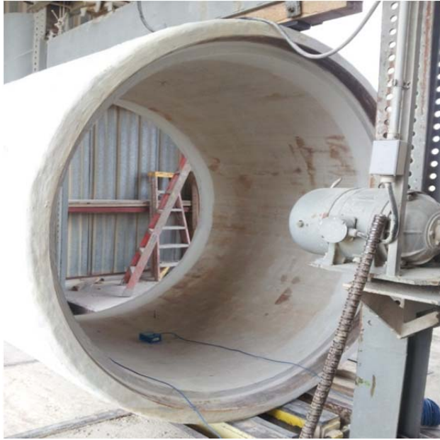
Figure 2.12 Loading the PCCP-ECP through top bearing
