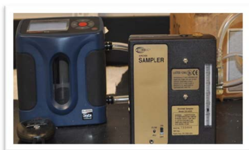
Figure 3.3 SKC Pump and Calibrator Used for Gas Volume Measurements (Source: Karanjekar, 2012)
