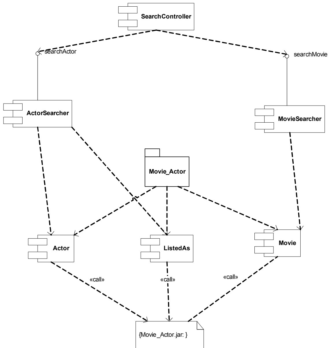
Figure 6.15 Component Diagram – Movie Actor Example
