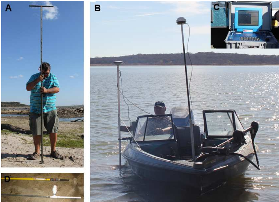
Figure 2-1 Data collection tools: images (A-D). Image A shows a Dutch auger with gouge attachment. Image B shows the boat used for bathymetry data collection. In this image the GPS receiver is pole mounted over the transducer and is located on the starboard side, and the WAAS beacon is pole mounted on the bow. Image C shows the SurveyCase SC-200™, and D shows sampling tools.
