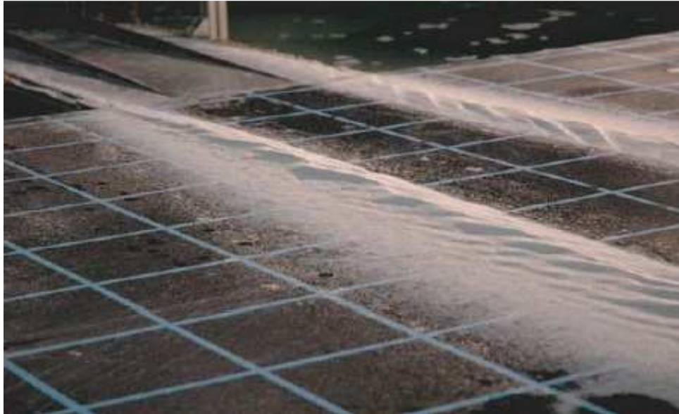
Figure 4-2 Rowland's flume experiment with 1.9 cm/s settling velocity particles. Oblique view with 20 cm grid shows experimental levee sedimentation.
