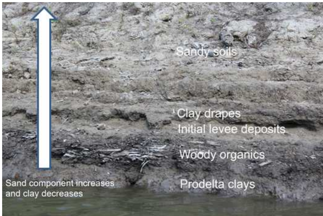
Figure 3-19 Typical progression of levee facies. Image is of the northern levee about 5,000 ft upstream of the mouth. Arrow shows direction of decreasing clay and increasing sand components.
