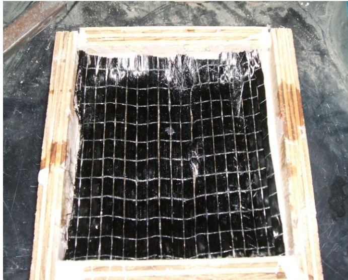
Figure 2.3 Tyfo SCH-41 composite material ready to be installed.
