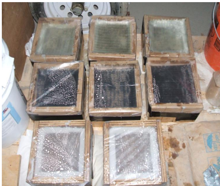
Figure 2.6 Concrete specimens completely taped and covered with polyethylene sheet.
