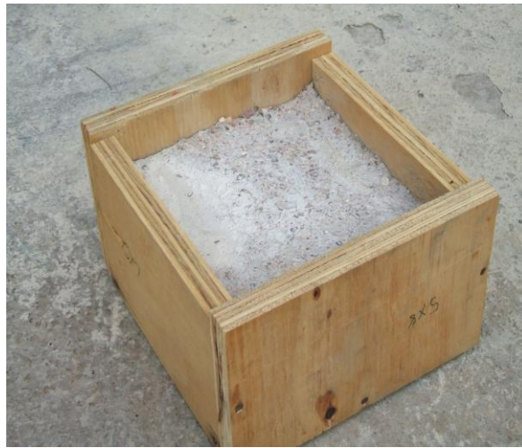
Figure 2.1 Cubic mold used to cast a concrete specimen.
