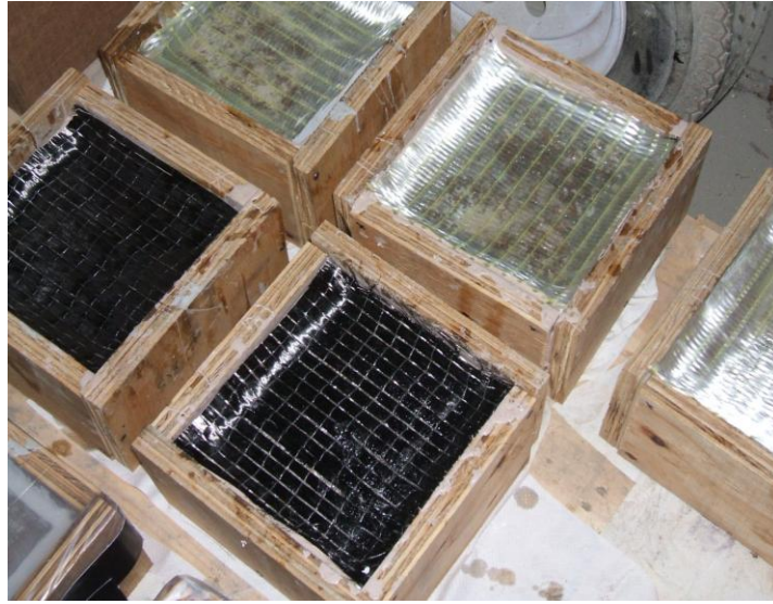
Figure 2.4 FRP installed on the concrete specimens.
