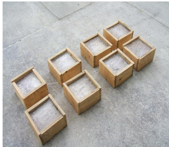
Figure 2.2 Concrete specimens before FRP installation.
