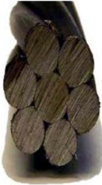
Figure 1.2 Prestressed strand used to reinforce concrete ( www.grin.com ).
