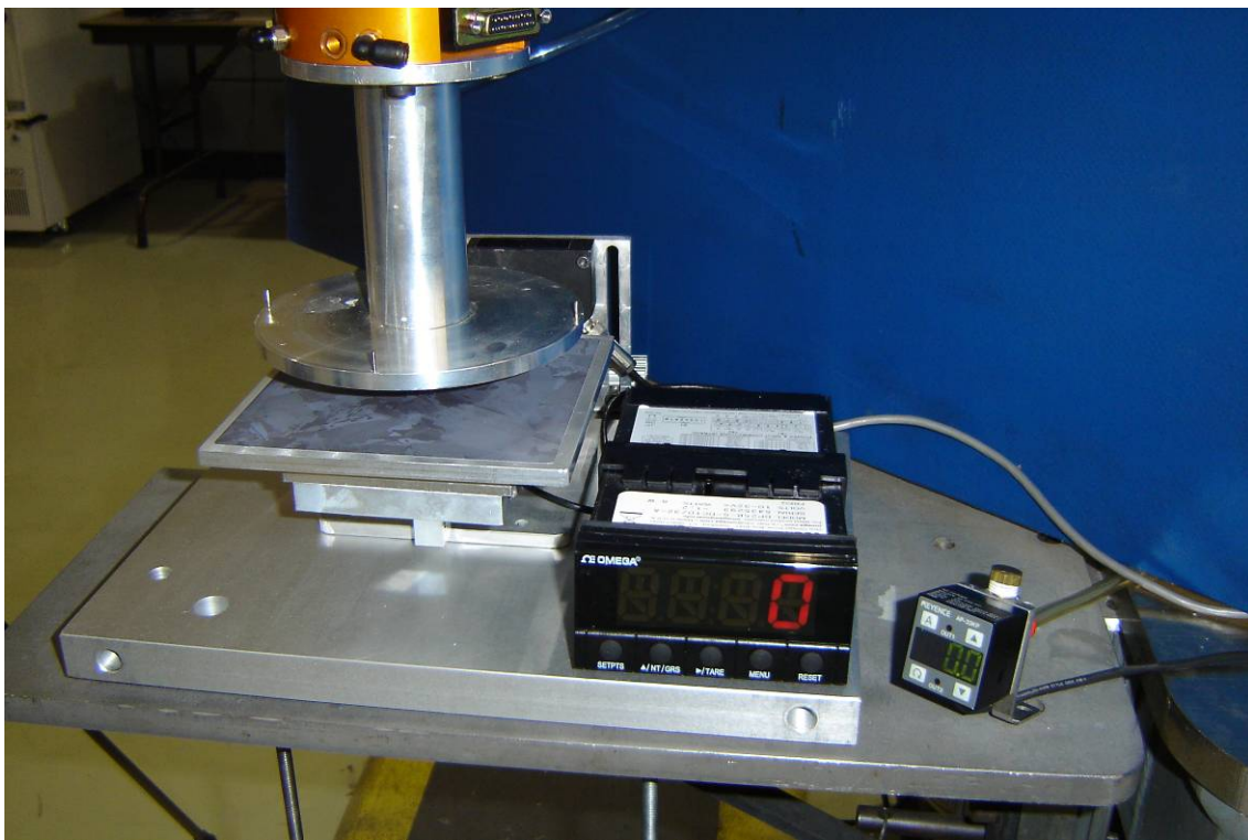
Figure 5.10 Net force vs. gap experiment apparatus
