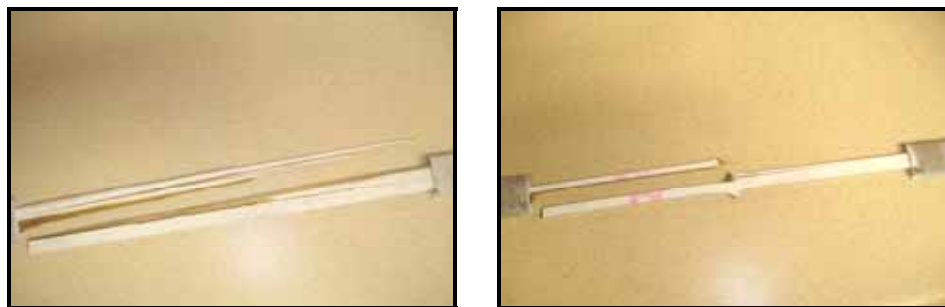
Figure 3.4 Typical Splitting Failure in Tensile Test – 12 in (304 mm) with node
