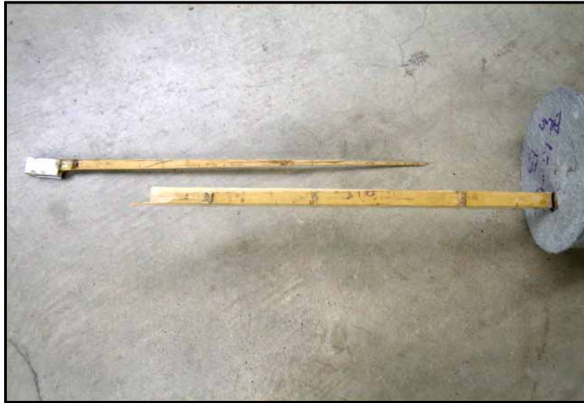
Figure 3.25 The Grip Failure of Pullout Test
