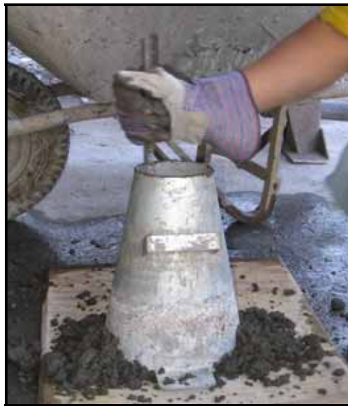
Figure 2.13 Tamping of Slump Test with Rod
