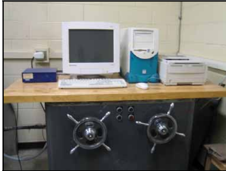
Figure 2.18 Data Collection with an Automatic Data Acquisition system
