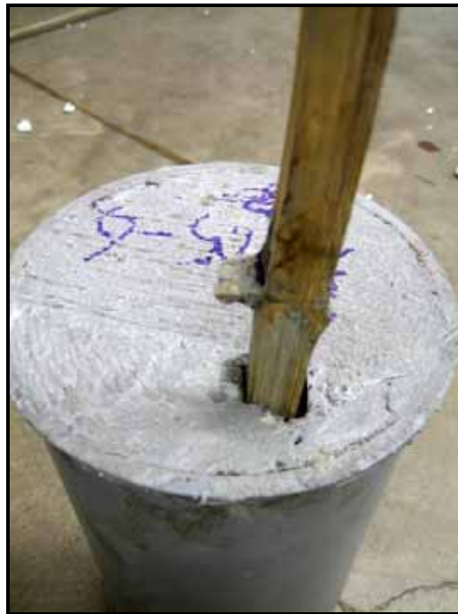
Figure 3.24 Pullout Failure Specimen
