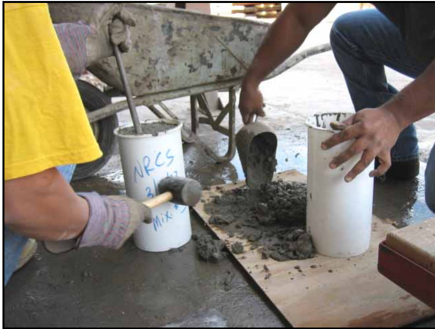
Figure 2.15 Motion of the rod and rubber mallet and pouring concrete
