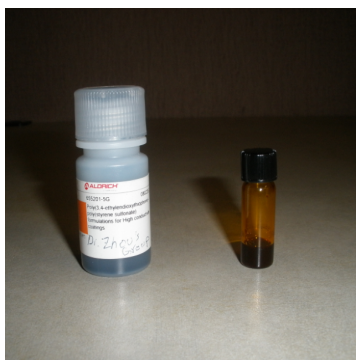
Figure 3.7 Picture showing PEDOT: PSS (left) and blend of P3HT and PCBM in chlorobenzene
