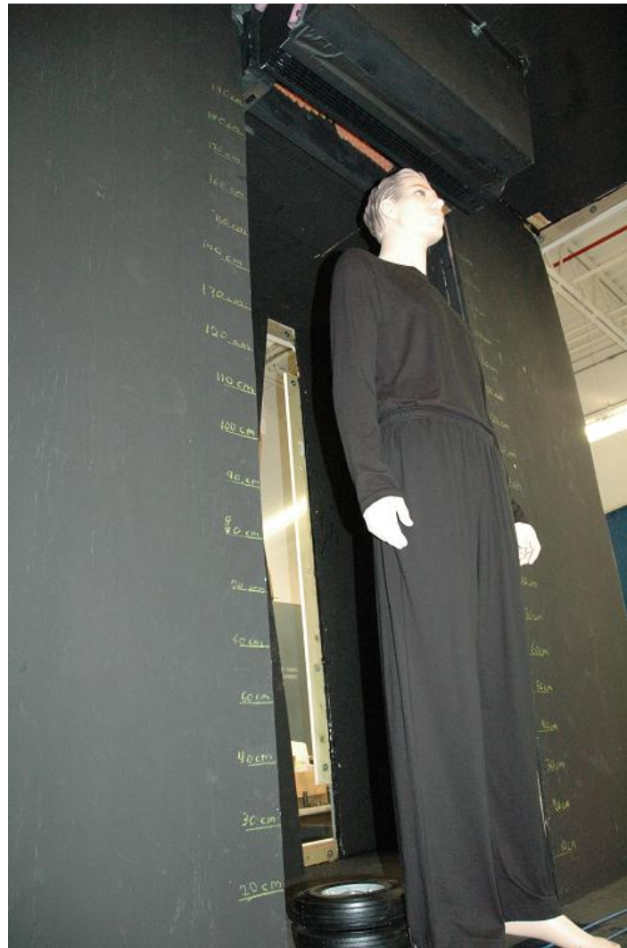
Figure 2.3 Photograph of air curtain mounted just ahead of the doorway with the mannequin
