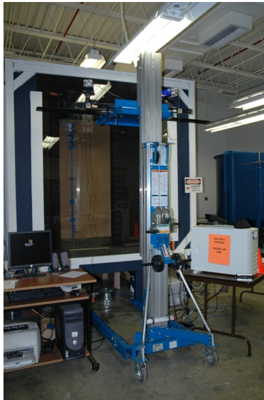
Figure 2.5 Photograph showing the lifting mechanism with the stereo cameras
