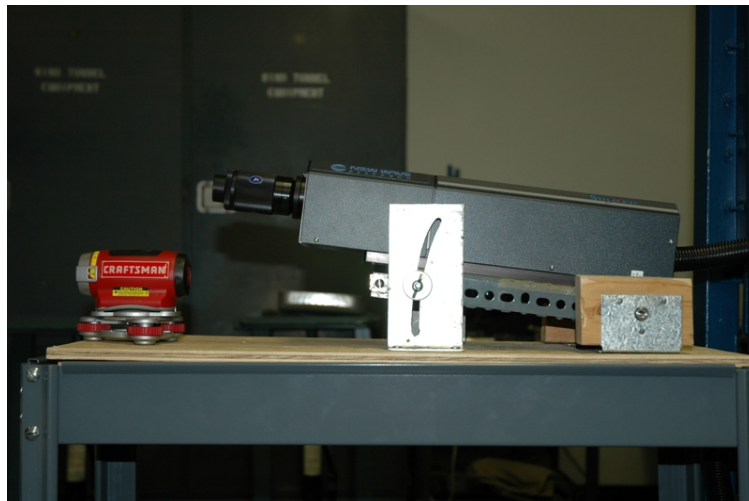
Figure 2.4 The precision laser level mounted ahead of the Nd:YAG laser
