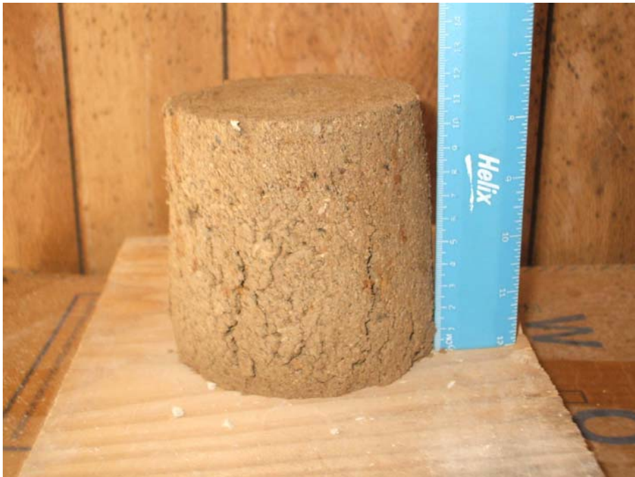
Figure A6 Limestone aggregate test sample after unconfined compression strength test
