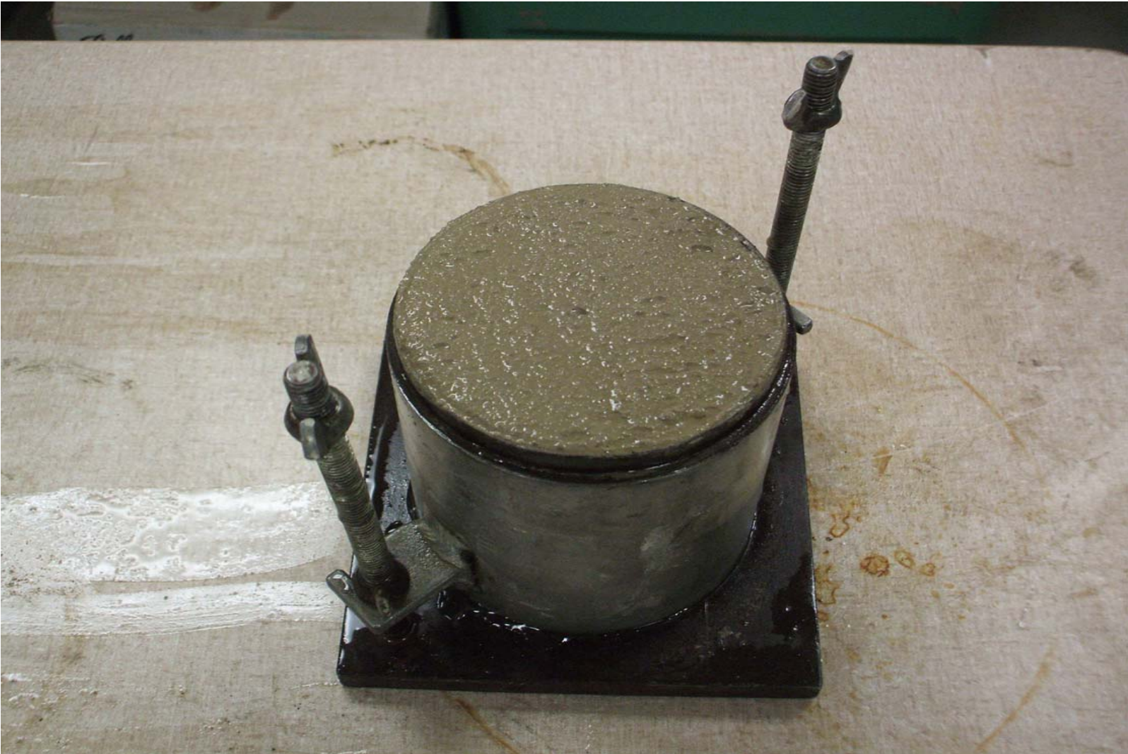
Figure 4.33 Compacted recycled concrete aggregate RC1 at wet density condition
