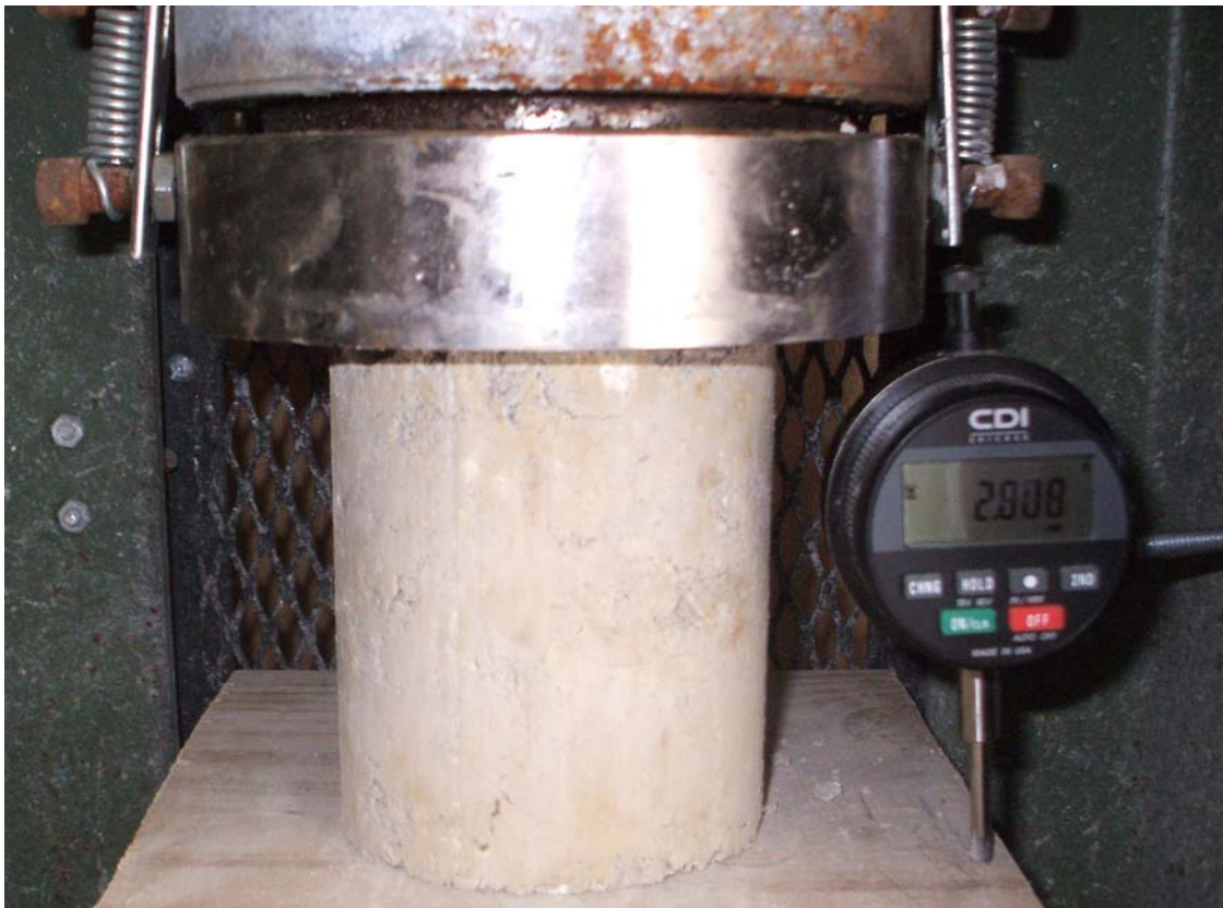
Figure 3.20 Four-inch diameter specimen in compression with digital displacement recorder
