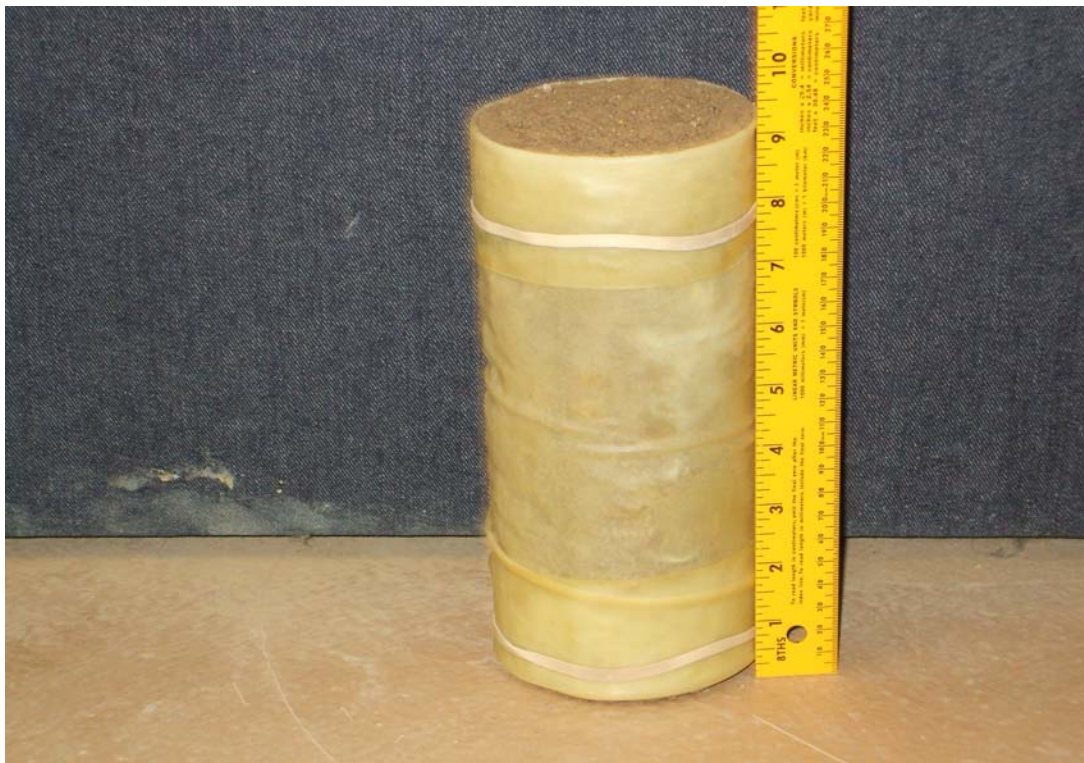
Figure A2 Secondary sample size chosen (101.6 mm diameter x 231.8 mm)
