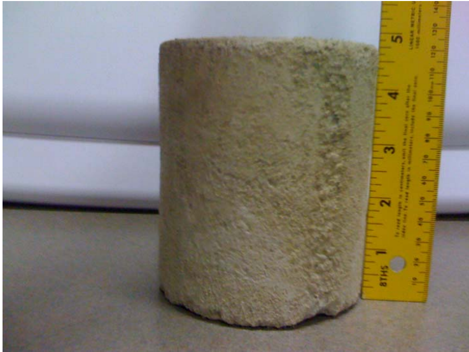
Figure A3 Samples size used for testing (101.6 mm diameter x 120.7 mm length)
