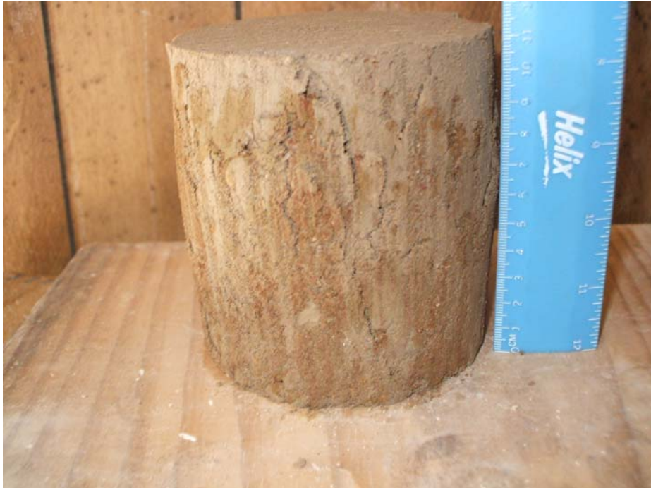
Figure A5 Recycled concrete aggregate RC2 after unconfined compression strength test
