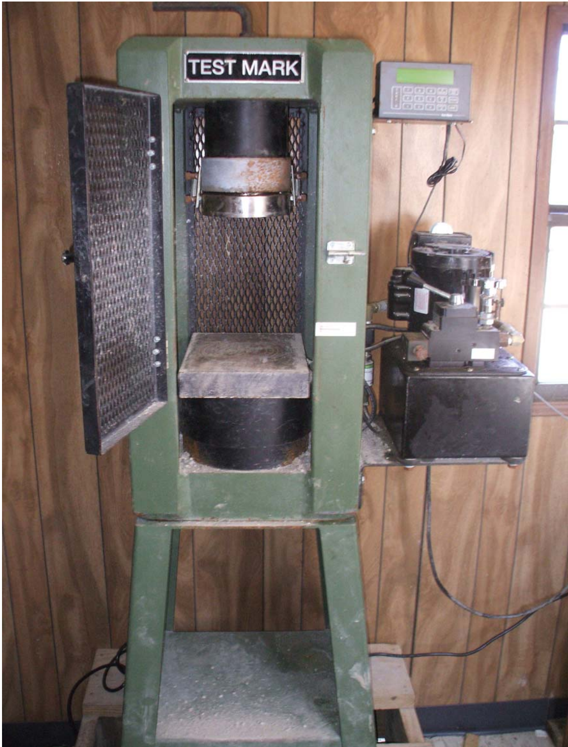
Figure 3.21 Test Mark CM-3000 compression machine with digital loading indicating system
