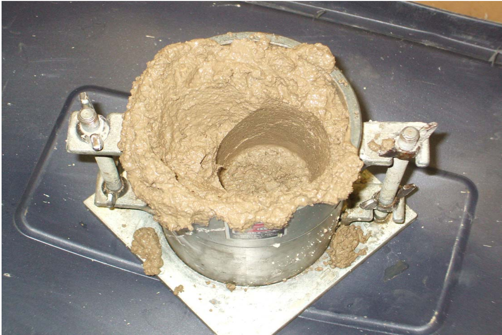
Figure 4.32 Recycled concrete aggregate RC1 at wet density condition during compaction
