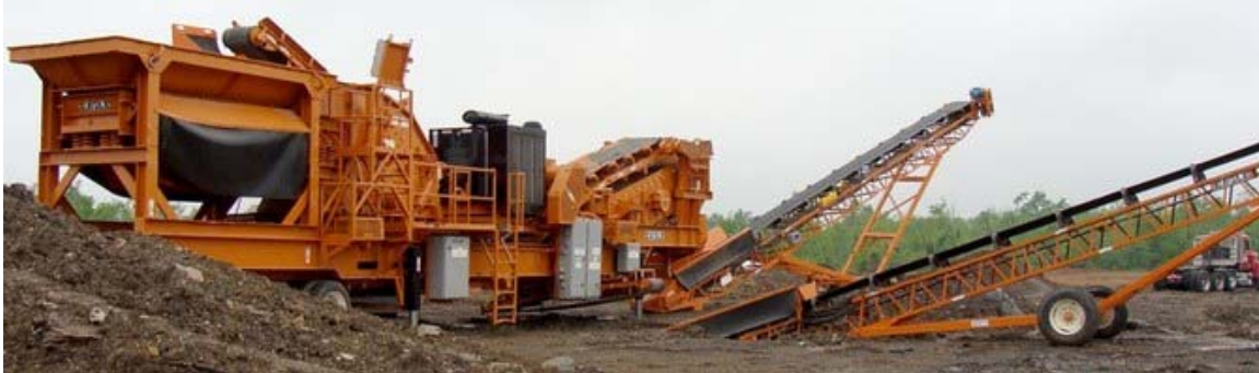
Figure B1 Portable and mobile crushing plant ( www.txlsm.com )
