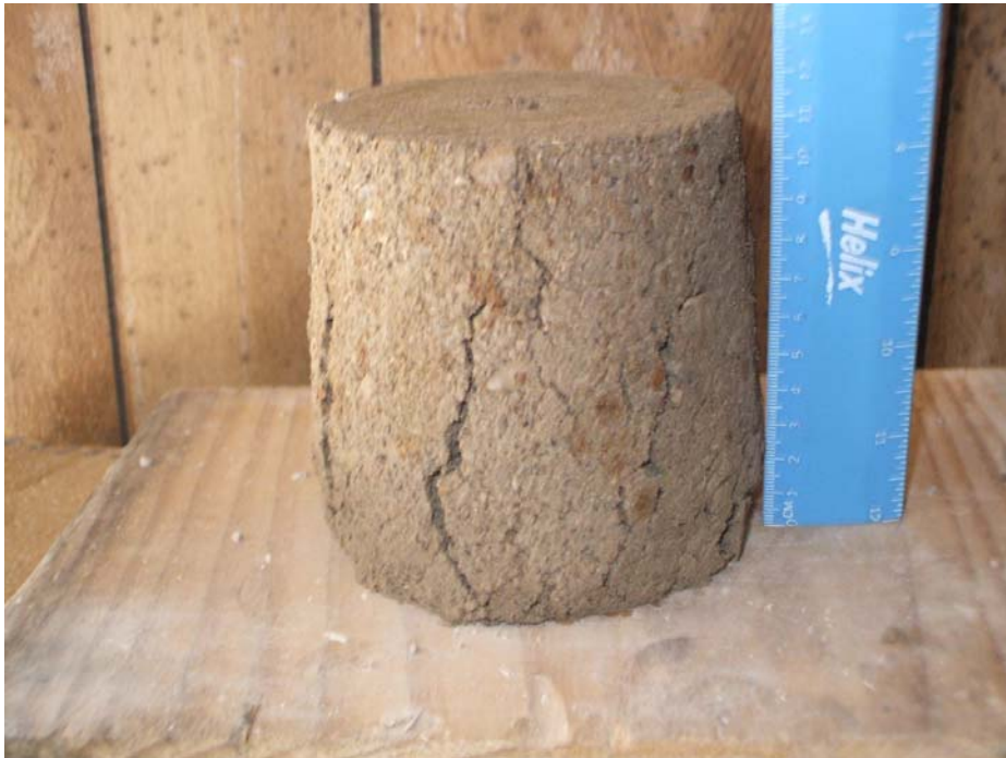
Figure A4 Recycled concrete aggregate RC1 after unconfined compression strength test
