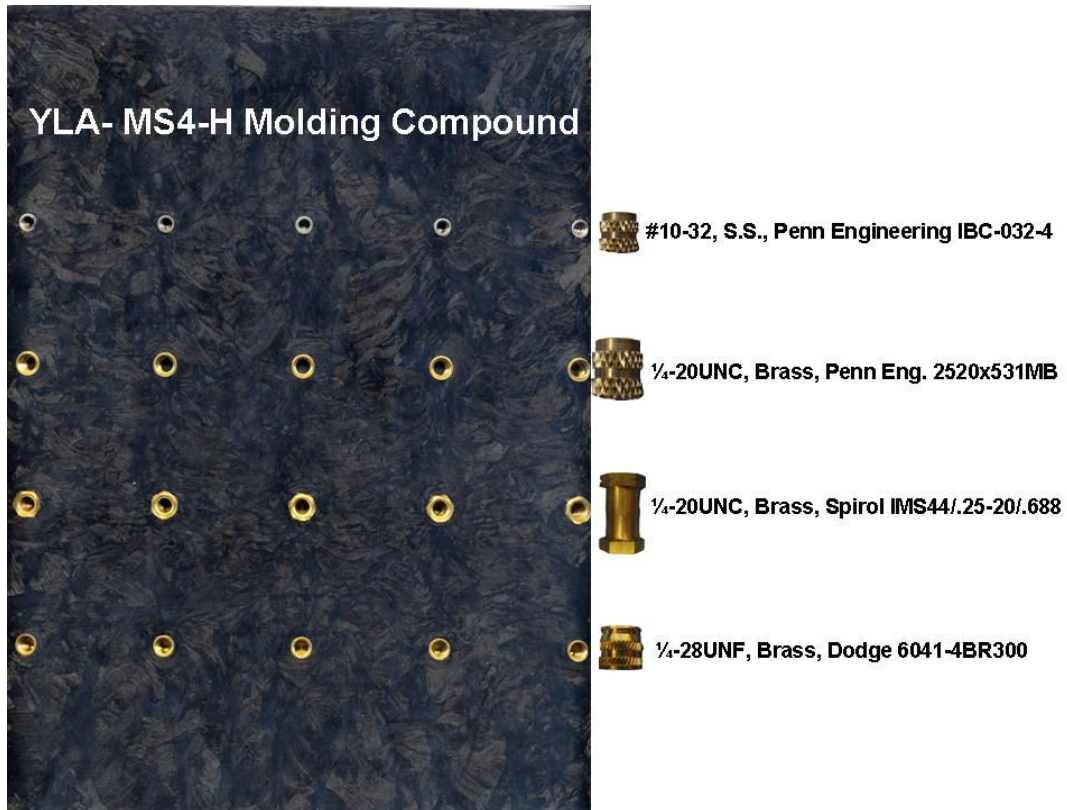
Figure 2.7- YLA MS-4H Molding Compound with Embedded Inserts
