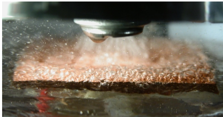
Figure 4.9. Image of spray cooling at 200 ml/min using the 30×30×3 mm heat spreader outputting 200 Watts. Vigorous boiling is observed at the perimeter of the heat spreader.
