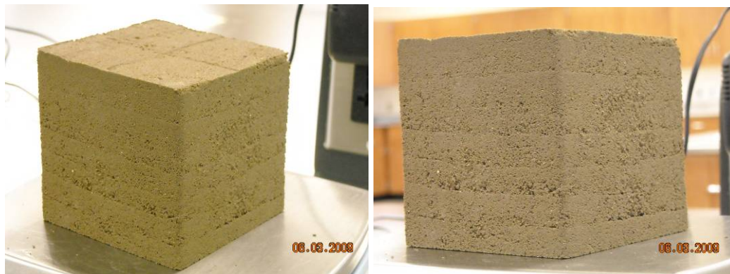
Figure 5.13 Typical layered SP-SC samples compacted using in-place tamping method.
