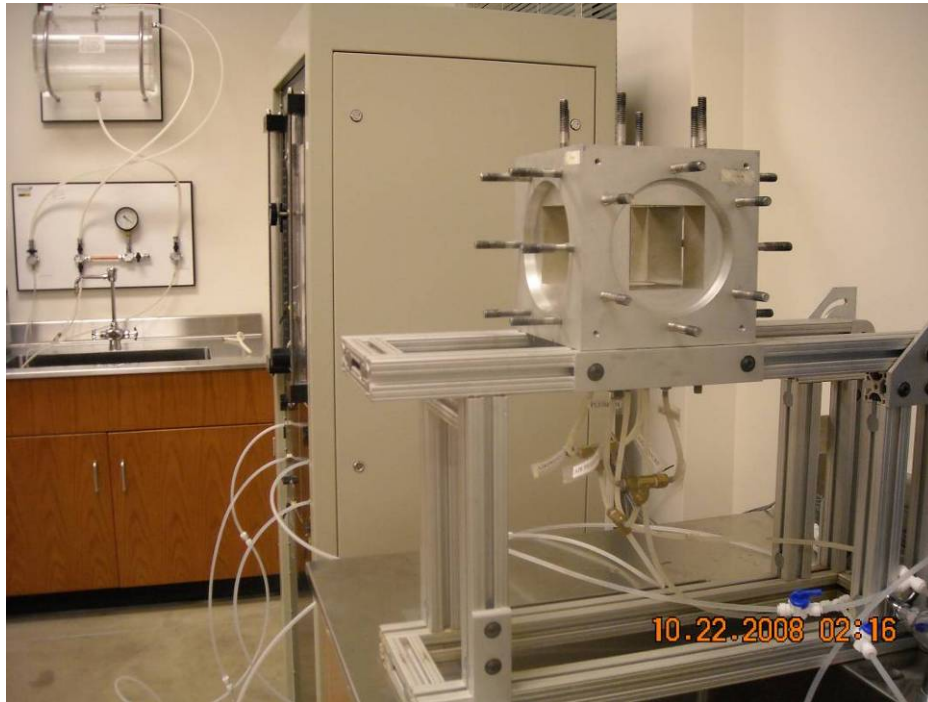
Figure 4.20 Cubical frame with the bottom assembly secured to the supporting frame.
