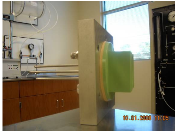
Figure 4.22 Top/lateral wall assembly with rubber membrane.
