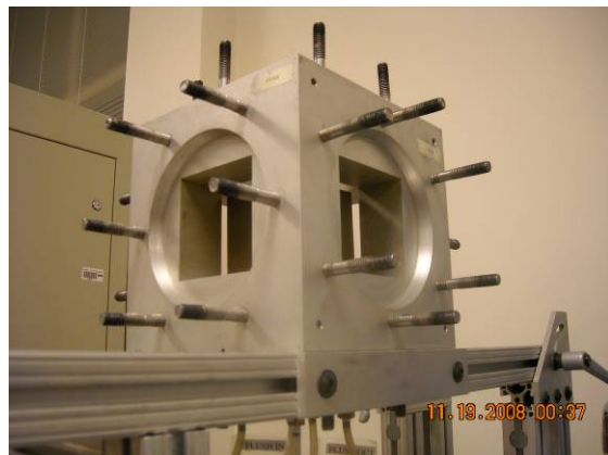
Figure 4.23 Sample into the cubical core frame.
