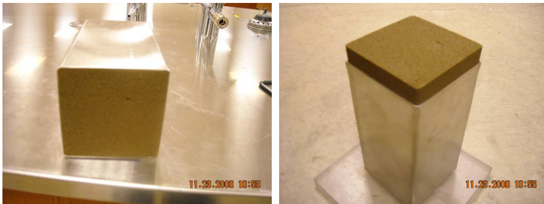
Figure 5.17 Homogeneous SP-SC sample compacted using static approach.
