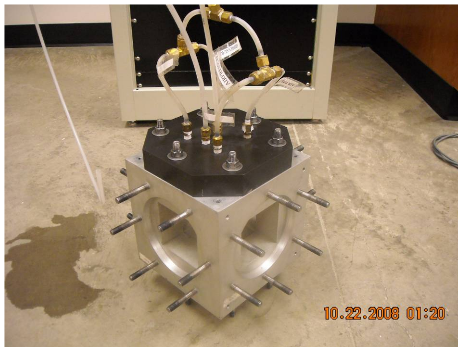
Figure 4.19 Cubical frame with the bottom assembly (shown upside down).
