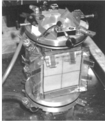
Figure 4.7 Cubical silty soil specimen with the upper and lower loading plate (Matsuoka et al., 2002).
