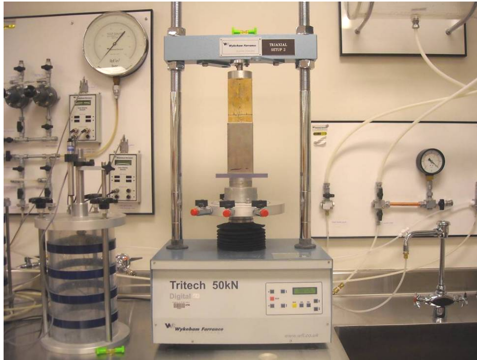
Figure 5.16 Static compaction using triaxial load frame.
