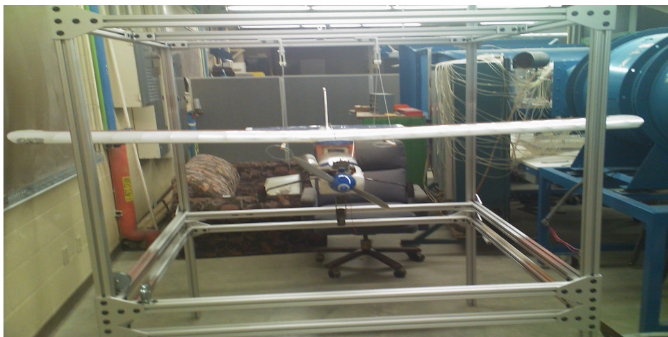
Figure 2.4. Experiment Setup for Moment of Inertia about Y-axis.
