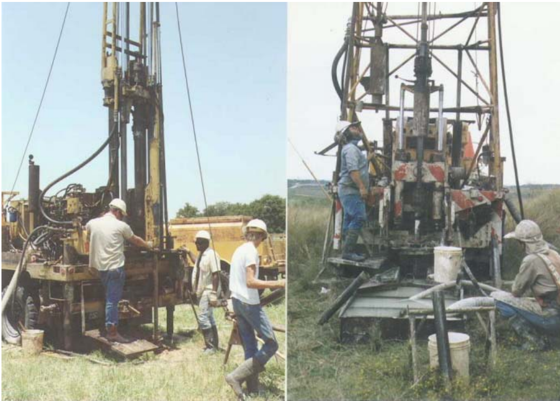
Figure 2.4 TCP Hammers – Fully Automatic on Left; Automatic Trip on Right (Geotechnical Manual, 2000)
