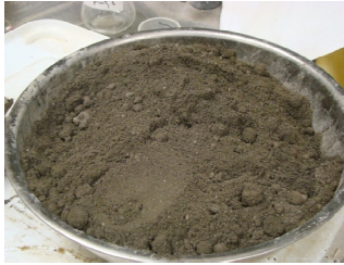
Soil mixed with lime after mellowing
