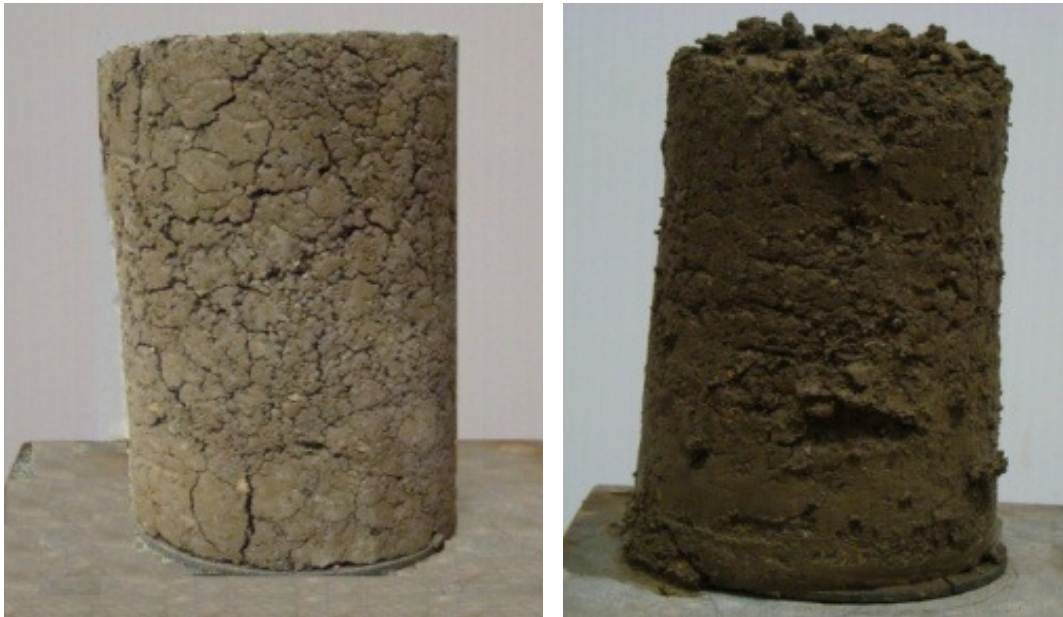
Figure 5.21 Changes in untreated Paris soil specimen with Wetting/Drying cycles a) At start b) After 1 wetting cycle c) After 1 drying cycle d) After 2 wetting cycles
