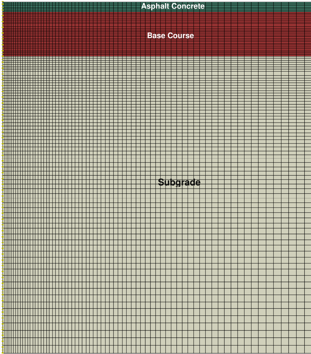
Figure 7.4 Selected mesh size for a typical section analyzed in this study
