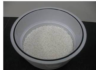
Desiccator containing \text{CaCl}_2
