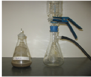
Soil sample saturated with \text{NH}_4\text{OAc}
