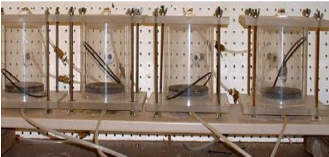
Figure 2.21 Cyclic wetting-drying setup
