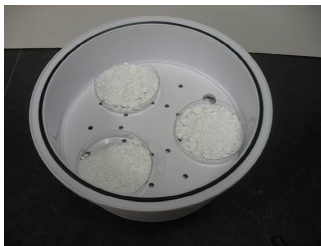
Desiccator containing \text{CaCl}_2 -EGME Solvate over \text{CaCl}_2
