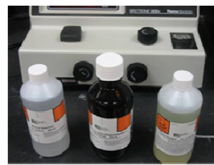
Colorimetric determination of ammonia concentration
