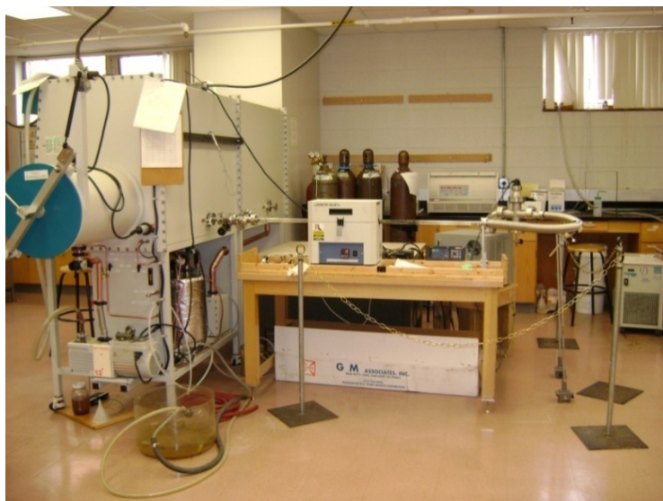
Figure 3.9 High vacuum set up connected with inert medium glove box.
