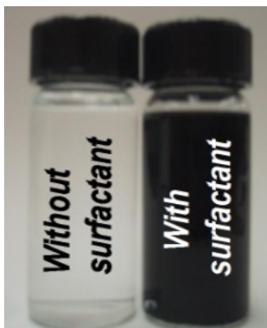
Figure 3.7 Particles in heptane solvent after milling.
