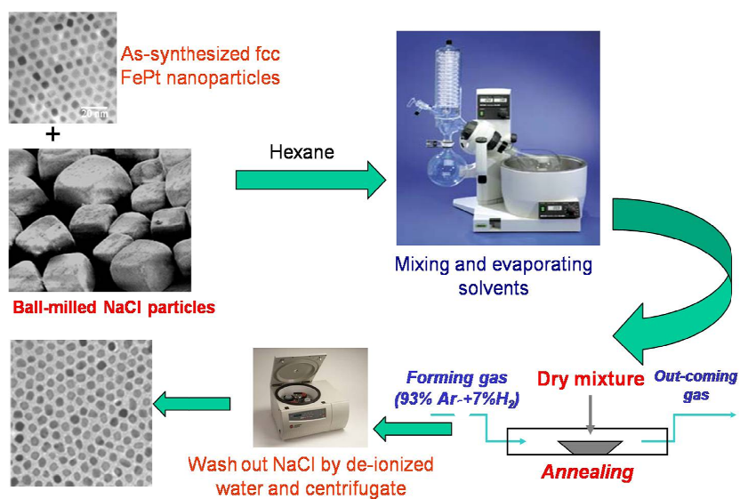
Figure 3.5 Schematic showing salt-matrix annealing technique.
