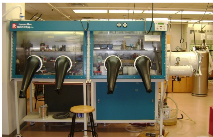
Figure 3.8 Glove box maintained in Ar gas environment to protect samples from oxidation during process and storage.
