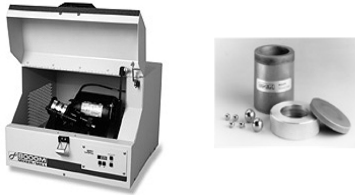
Figure 2.6 Spex 8000M Shaker mill and milling container along with balls.
