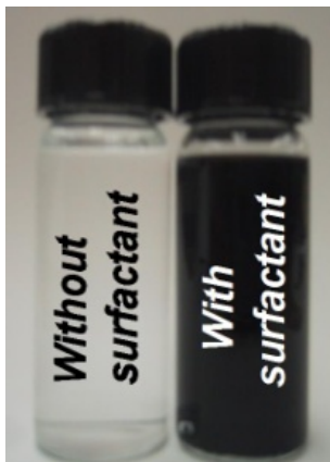
Figure 8.1 Particles in heptane solvent after milling.
